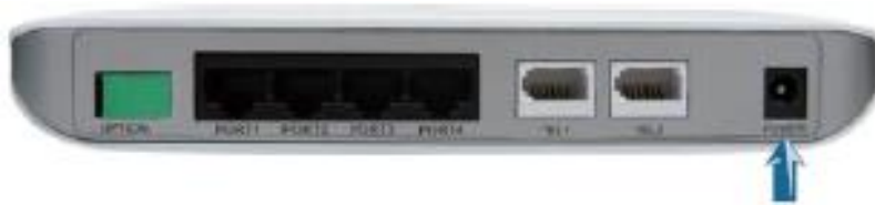
Figure 5 – Type 1 ONT showing ports and LEDs
