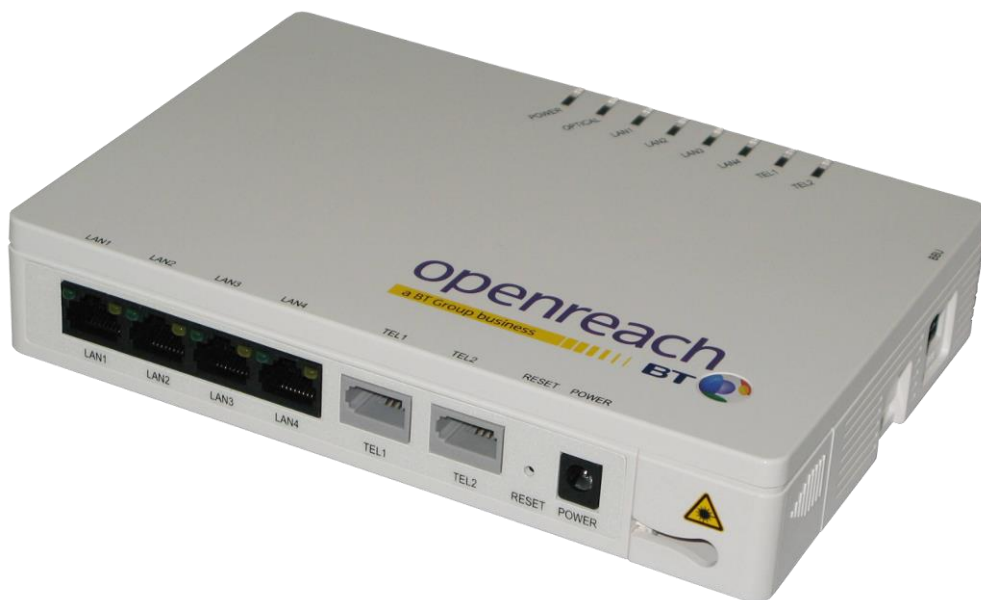
Figure 6– Type 2 ONT showing ports and LEDs
