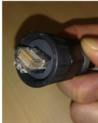
Required RJ45 connection from customer
