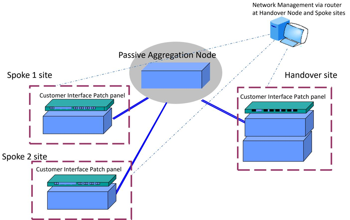
**Figure 1 Typical FSP3000 OSA Aggregated Hub and Spoke configuration**
