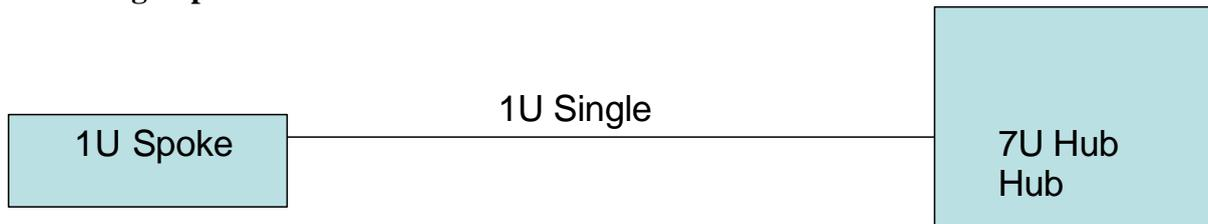
For this configuration, the term “single” is used to indicate that 1U high FSP3000 shelves are deployed without DWDM filters and will only support a single channel.
