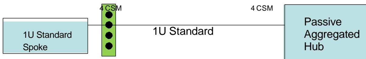
A single 4-channel filter (4CSM) is fitted as standard to this spoke bearer, therefore this service will support (non-traffic affecting) channel growth to 4 wavelengths.
