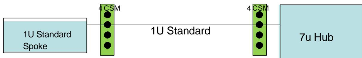
A single 4-channel filter (4CSM) is fitted as standard to this spoke bearer, therefore this service will support (non-traffic affecting) channel growth to 4 wavelengths.
