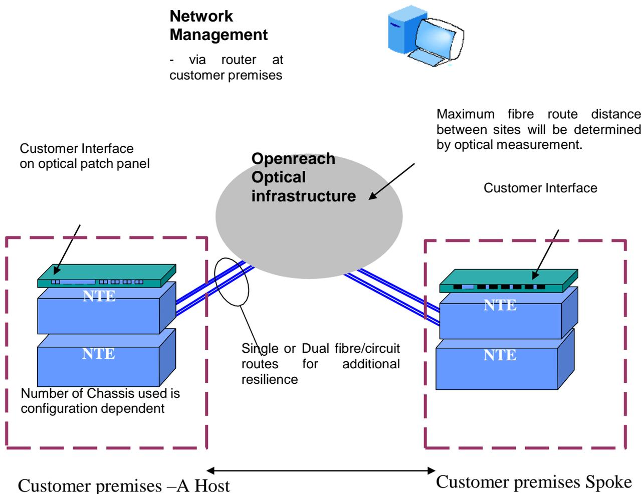
The Maximum distance supported on FSP 3000 will be dependent on fibre route distance and card/filter configuration.
