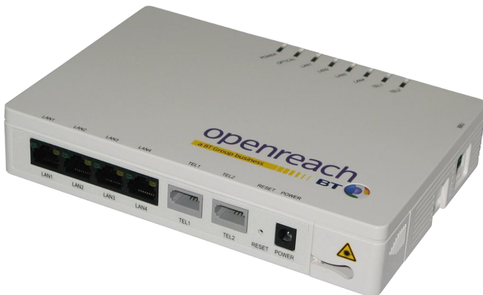
Figure 6– Type 2 ONT showing ports and LEDs
