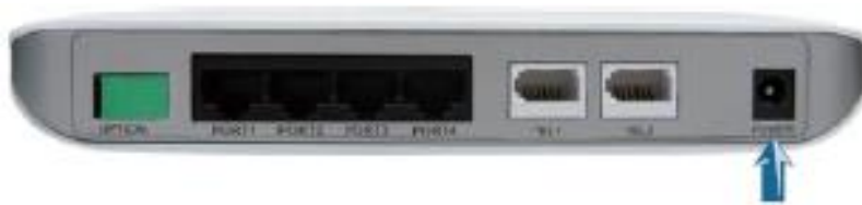
Figure 5 – Type 1 ONT showing ports and LEDs
