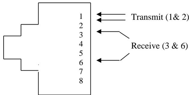
*Figure 4. WES/WEES/WES-LA 10 NTE RJ45 Connector Pin Out Connections*
